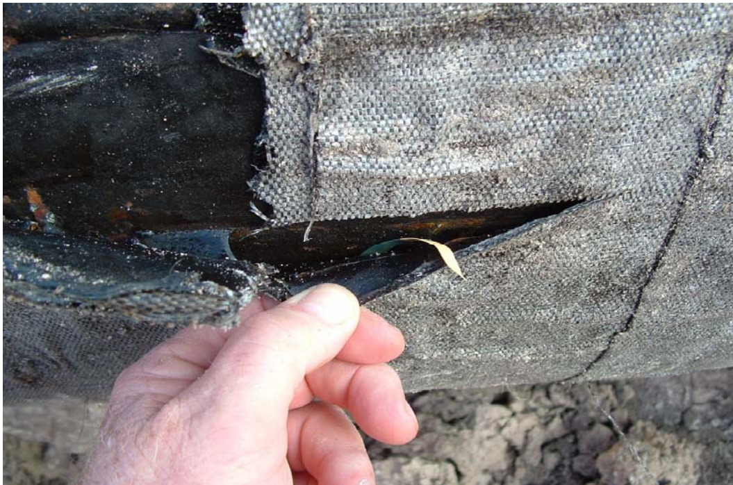
Photo #1 - 12" diameter pipe with corrosion on FBE coated pipe. This pipe had a large boulder setting on top of the pipe shielding CP.
