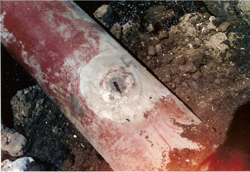
Photo #1 - 12" diameter pipe with corrosion on FBE coated pipe. This pipe had a large boulder setting on top of the pipe shielding CP.
