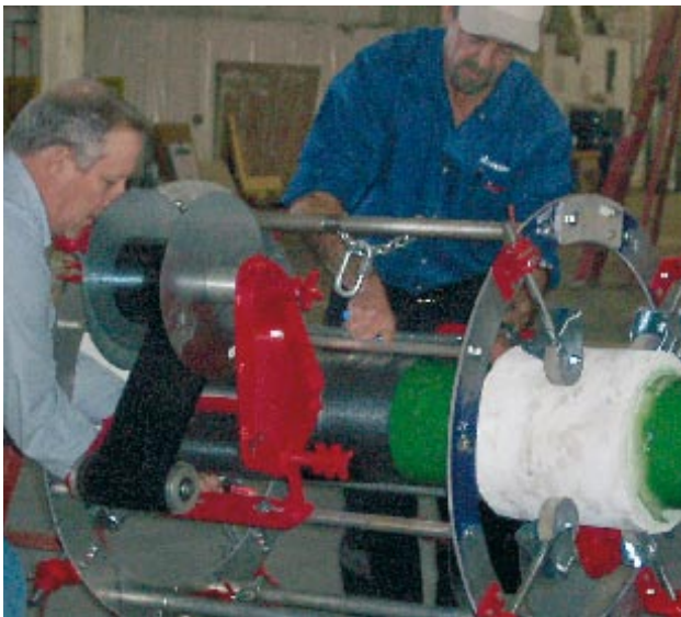
Figure 2. Demonstration of offshore applicator. Typical application takes less than two minutes.
